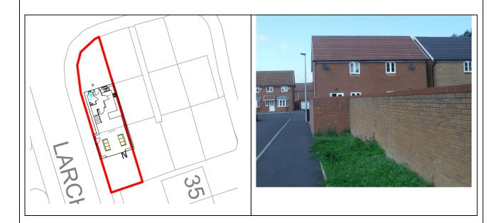
1.3 The proposed extension projects 4.2m from the main back wall of the house and extends across the full width of the garden projecting 0.67m beyond the side elevation of the house. It will have a pitched roof and have a set of French doors at ground floor level and two windows at first floor serving the two bedrooms.
